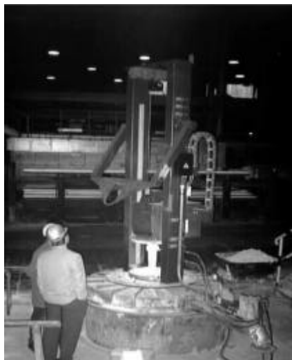
Figure 6 - FDU/MT Argon stirring unit in an induction furnace
