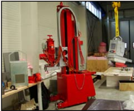
Pyrotek Metallurgics STAR degassing unit, now built in Europe
