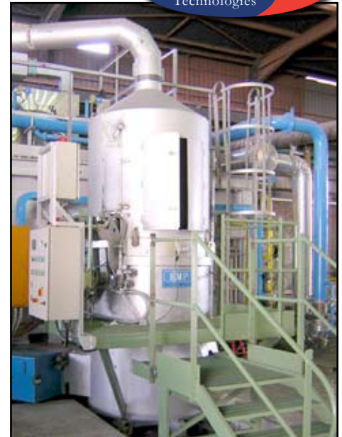
The EMP system provides a highly effective stirring solution for aluminium in a static furnace bath while allowing various scrap and other elemental additions to be loaded in a uniquely efficient way. The system incorporates patented EMP technologies within a closed loop comprising an EMP pump, based on a linear motor and an EMP chargewell.
