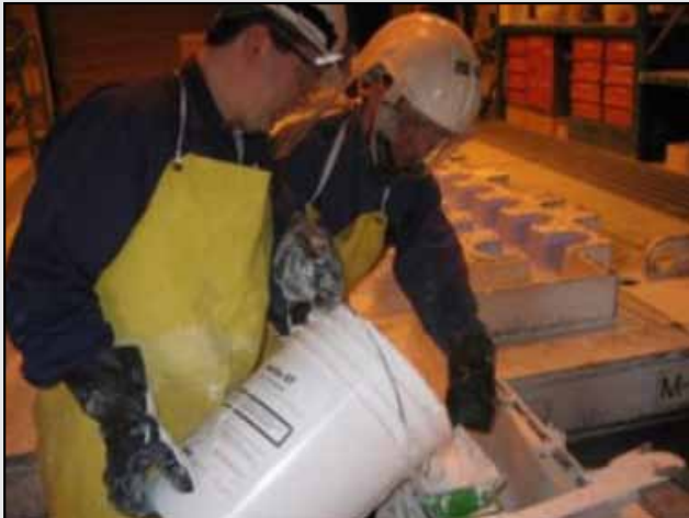
After mixing and pouring Pyrotek's Wollite in a liquid state, it expands and solidifies within a matter of minutes.
