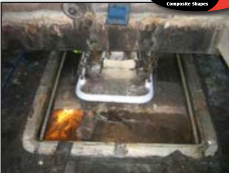
RFM skim dam in operation
